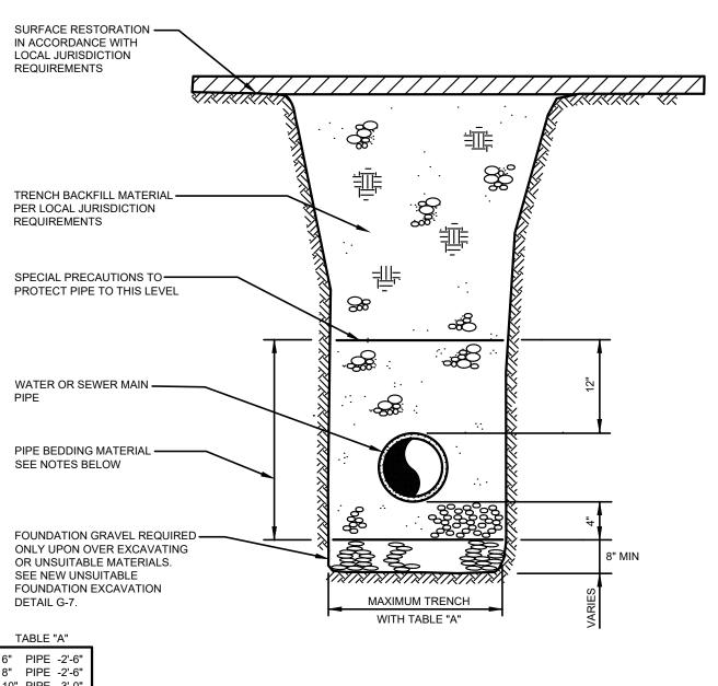
6" PIPE -2'-6" 8" PIPE -2'-6" 10" PIPE -3'-0" 12" PIPE -3'-6" 16" PIPE -3'-6" 18" PIPE -4'-0" 24" PIPE -4'-0"
